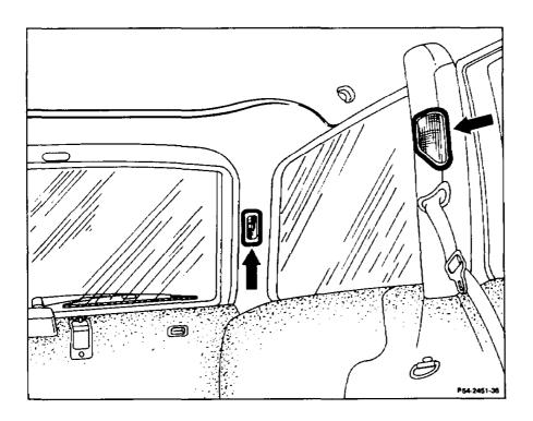
Dome lamp ...... unclip at the side marked with arrow, clip into place.
