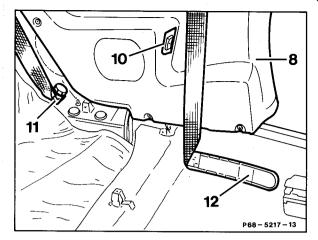
Seat belt extender ..... extend forward and pull off guide (9), install.
