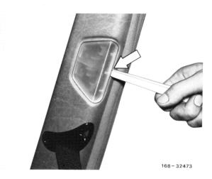
3 Disengage holding clamp with plastic wedge and remove trim.
