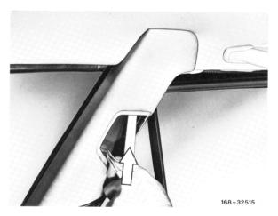
4 Unscrew belt end fitting on vehicle floor and remove trim.
