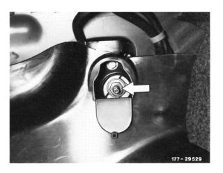
Note: Hold the shaft of the gear unit by means of an open-end wrench (6 mm) at the place provided for this purpose to make sure that the shaft will not rotate at the same time.
