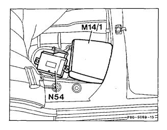
Rear seat bench or right individual rear seat .... remove, install. Electrical connector ...... disconnect, connect. Nuts ..... unscrew, tighten. Control unit (N54) ..... remove, install.
