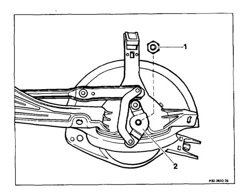
Nut (1) on wiper motor shaft ...... unscrew, screw on, 19 Nm. Crank arm (2) ..... press off, fit on.
