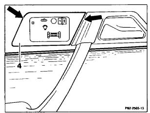
4 Unscrew switch (arrows) and detach plug connectors of wiring harness from switch.
