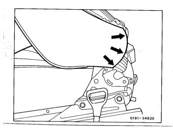
6 Separate rivets on backrest frame and remove vacuum switch with holder from backrest frame.
