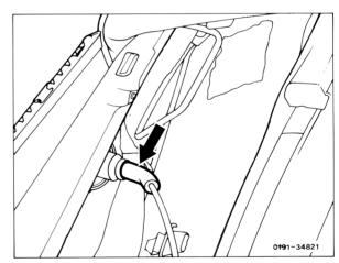
5 Disengage lining laterally from backrest fitting, below.
