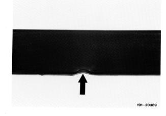
The guide rail is deformed. The seat can no longer be properly adjusted.
